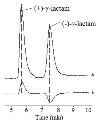
**Figure 2.** Chromatograms obtained from the (rac)- $\gamma$ -lactam enantiomers on Chiralcel OD-H. Conditions: mobile phase, *n*-hexane–isopropanol (80:20, v/v); flow rate, 1.0 mL/min; column temperature, 30°C; detection wavelength, 254 nm; UV detection (A); and optical rotation detection (B).
