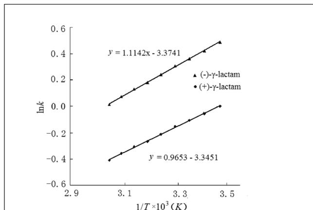
Figure 3. Plot of  $\ln k$  versus  $1/T$ . Conditions: Mobile phase, *n*-hexane–isopropanol (80:20, v/v); flow rate, 1.0 mL/min; UV detection wavelength, 254 nm.
